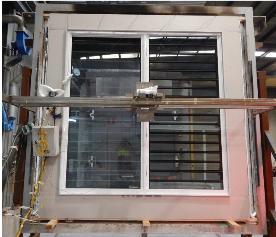
Figure 19 Unexposed face of the specimen at the end of the test
