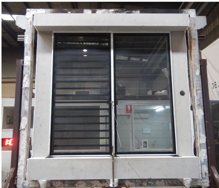
Figure 20 Exposed face of the specimen at the end of the test
